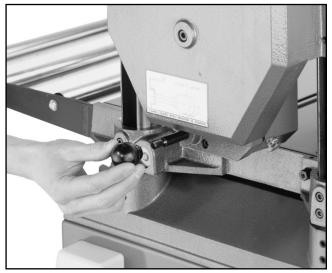
Figure 4. Installing speed change knob.
